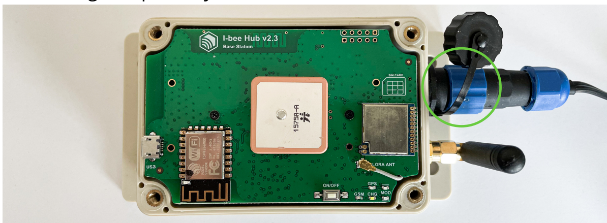
Picture 11 - connecting the power source
